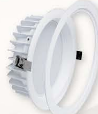
Downlight LED 30W 4000K 220-260mm Fascia, 200-245mm Cut Out 3000 lumens, dimmable, IC-F, IP40. ADL30W220-260 - Q5070280
