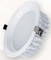
Downlight LED 16W/20W 4000K 192mm Fascia, 175mm Cut Out Dual power, 1700/2300 lumens, dimmable, IC-F, IP40. ADL20W192 - Q5070270
