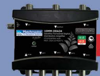
4-Way Digital Distribution Amplifier with Backfeed and 4G/5G Filter (Economy) 3 separate inputs; satellite, terrestrial (includes FM) and backfeed, powering for the satellite LNB, 4G/5G LTE filtering, power supply, 18V DC 1A regulated. 10MM-DDA34 - 43442870
