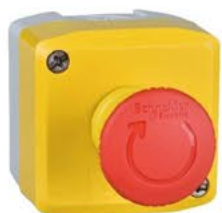
Harmony XALD, XALK, Complete Control Station Plastic, yellow lid, 1 red mushroom push button 40mm, turn to release, 2NC XALK178F - 68120240
