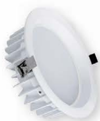
Downlight LED 16W/20W 4000K 192mm Fascia, 175mm Cut Out Dual power, 1700/2300 lumens, dimmable, IC-F, IP40. ADL20W192 - Q5070270
