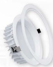
Downlight LED 30W 4000K 220-260mm Fascia, 200-245mm Cut Out 3000 lumens, dimmable, IC-F, IP40. ADL30W220-260 - Q5070280
