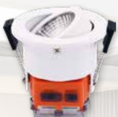
Tiltable Dual Power 4W/8W Downlight 90mm 3000K/4000K 75mm Cut Out 400-850 lumens, dimmable, IP65, 80+ CRI. ADL90DP - Q5071100
