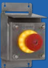
Emergency Stop Twist to Release Mechanical eye indication, with 24V AC/DC luminous ring, 1x self-monitoring contact & 1x N/C contact block IP66/67 304 SS enclosure with sloping lid, welded mounting feet & single 20mm entry. PSN*NZ0762. 2342025 - 55815940
