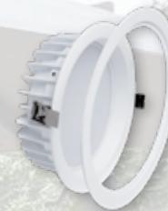
30W Downlight 220-260mm 4000K 200-245mm Cut Out 3000 lumens, dimmable, IC-F, IP40. ADL30W220-260 - Q5070280
